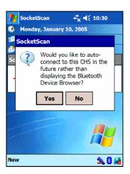
7. Your device will automatically connect to the CHS. If a passkey is requested, enter 1234. To indicate the connection, the CHS will beep once, and the SocketScan icon will change to show an image of the scanner.
